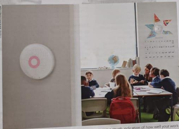
AND BREATHE Carbon dioxide (CO 2 ) monitors can give a rough indication of how well your workplace ventilation – whether it's via an open door or a full-on mechanical system – is working.
